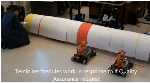
Fig. 7. Hardware demonstration of Tercio where two KUKA Youbots build a mock airplane fuselage alongside a human quality assurance agent.
